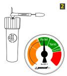
Remove the cover from the injection valve and insert the pump with the lever lowered. Lift the lever and pump pressure until the indicator's needle reaches the corresponding green zone (paddle or tennis)\*. Lower the lever, remove the pump (if necessary, remove any extra pressure by pressing the inside of the valve) and replace the cover.
